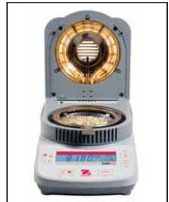
The OHAUS MB23 comes with an infrared heating element, while the MB25 uses halogen technology
